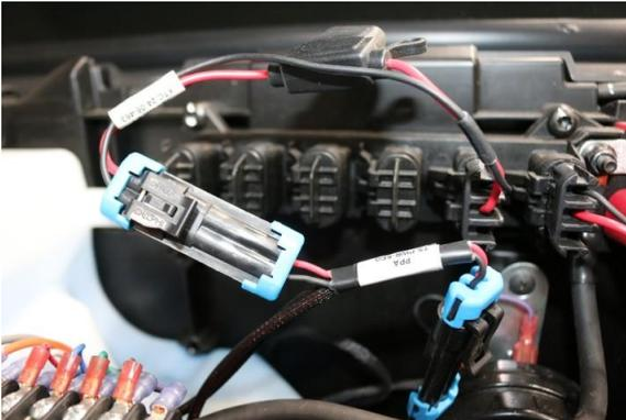
5. Run the green cable to the right side and the yellow to the left side with the front turn system harness.
