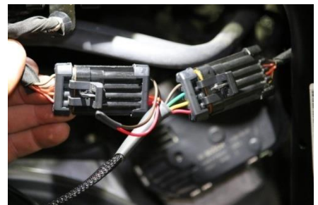
XTC Harness connector installed
