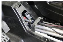
4. Plug rear Harness into OEM Connector - Unplug wire harness at rear left side and connect our harness, see photo below. (Note: There is a Red and Brown power wire provided for an optional license plate light). Run the rest of the harness to the rear lights, Green goes to right light and Yellow goes to Left. You may leave the factory rear harness in or remove it.
