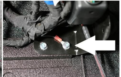
Run the power wire down the slot on the right side and reinstall the fuse cover. Remount the fuse box and using the mounting screw attach the black ground wire as shown.
