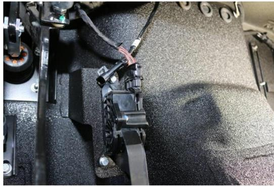
5. Mount the Control Unit as shown under the grommets using two self-tapping screws provided and Plug the Rear Harness in.
