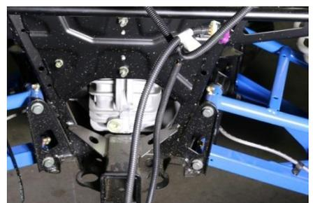
4. Unroll the long rear cable, starting with the 4-pin connector run the cable from the rear of the car over the OEM light harness connector down to the inside center tunnel and up the fire wall through the hole in the fire wall.
