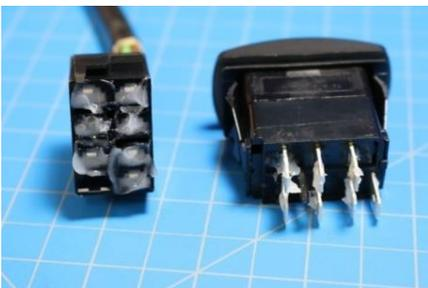
11. Install Horn/Hazard Switch - Using a new sharp razor, cut out switch rectangle. Do not over cut, try inserting switch and trim as necessary. It helps to rock the razor to cut. Run 10-pin connector through cutout and apply grease discussed above to both the terminals on the Horn switch and the 10-pin connector and insert in panel.
