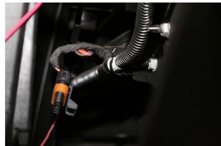
4. **Run Rear Harness** – Remove the seats and center plastic console. Starting at the rear run the long harness with the single 4 Pin Connector through the center of the car up the outside of the firewall through the rubber grommet to the control box and plug in. **Secure cable using the supplied cable tie's making sure to keep the harness away from any Hot or Moving parts.**
