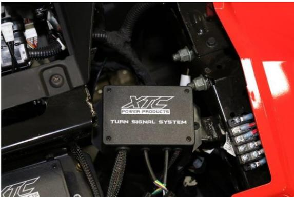
3. **Plug Rear Harness into OEM Ride Command 8 pin Connector** - Unplug the wire harness at the rear left side and connect our harness inline. (Note: There is a Red and Brown power wire provided for an optional license plate light). **TSS-POL-RC3** fits cars with third brake light. Reach into the rear and unplug the center brake light, run the 4-pin connector to the third brake light and plug in.
