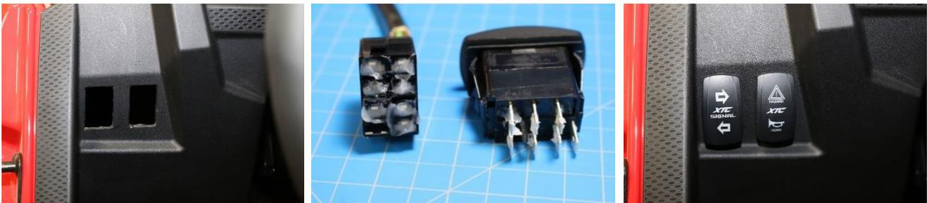
**Dielectric Grease** - LED flashers by design take very little current to activate. When water gets on the dash and lands on the top of the switch, it can trickle to the connector causing it to activate the flasher by using the switches LED indicator, the system will continue to operate and does not hurt the system but will continue clicking until the switch terminals dry. Just like the OEM we recommend using Dielectric Grease on all switch
