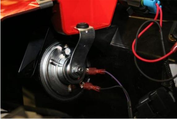
8. **Run power** – Run Fused power wire through the grommet and attach the red wire to the left accessory stud under the hood and ground to the black wire center, mount fuse to screw.
