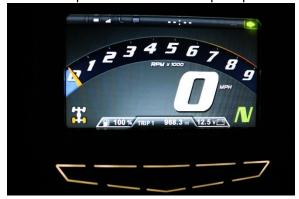
The TSS-POL-INS Polaris Indicator Kit does not work on the new Analog/Digital Instrument Cluster that is in the General, Turbo S and 2018 Ranger New Body Style. Polaris controls these with the ECU and is not reliable.
