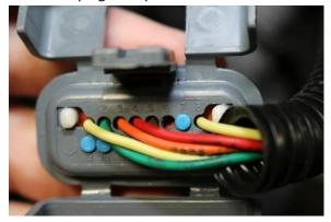
5. Insert Terminal – Insert the Terminal into hole 6, re-install plastic locking cover and snap cover closed.
