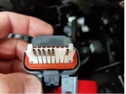
4. **Remove Plug** – Using a pair of needle nose pliers remove the plug from port 6 shown.
