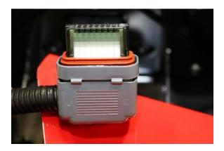
3. **Remove Connector Lock** – Using a small screw driver push in on both sides of the connector at the white locking tabs shown below and slide smoked colored cover off exposing the pin terminals.
