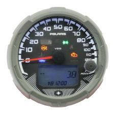
**Note:** If you have one of the newer LED clusters that has separate Left and Right Arrows, the pilot cannot be used, they require left and right signal. This is accomplished with our adapter part number TSS-POL-INS.
