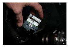
5. Remove Plug – Using a pair of needle nose pliers remove the plug from wire port 8 and insert the Terminal into it
