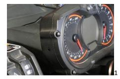
3. Unplug Connector – From the rear of the Instrument Cluster by pushing on tab while pulling it off
