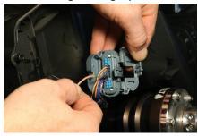
6. Close Cover – Run our adapter cord along side the OEM harness and snap shut, re-install plastic locking cover
