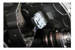
4. Remove Connector Lock – Using a small screw driver push in on both sides of the white connector and slide lock off.
