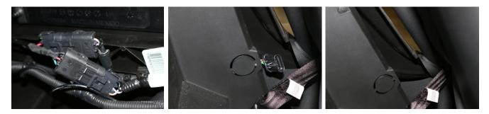
**Run the other end** - of the rear harness to the front kick panel. The plastic has a perforated circle behind the driver's seat or rear seat behind the driver on the MAX, at this location you can push the rear harness single connector through the plastic gap to the passenger compartment, follow the frame along the driver's side, the harness can be hidden in the side panels and goes up behind the removed kick panel over the frame rail.
