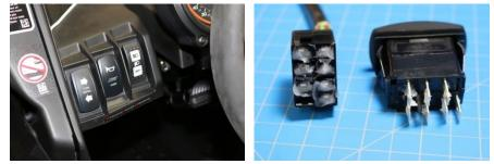
**9.** Install Hazard/Horn Switch - - Remove one of the switch blanks and run our 10-pin switch connector through the opening, grease the terminals with the supplied grease and attach to Hazard/Horn switch and insert the switch into the opening.
