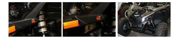
6. **Install Front Harness** - Starting from behind the radiator run the short front harness's 4 pin connector through center rubber seal along the factory wiring, from the inside pull it through and run it over the brake mount and steering mount over to control box, plug into the control box mounted on the kick panel.
