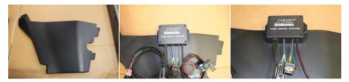
3. Run the Rear Harness - Starting at the rear driver's side light harness, these connections are on the plastic wall in the front engine area, take the end of the cable with two connectors on it and run it from the OEM Rear Light Harness on the Driver's side to the OEM Rear Light Harness on the Passenger side, follow the factory wiring, unplug both harness and install our harness into the factory harness. Secure using the supplied cable ties
