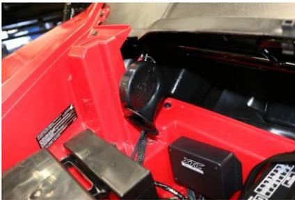
4. Install the Rear Harness, under the rear of the car is a 6-way connector, unplug the connector by pushing in on the tab on the left side facing the front of the car. Plug our rear harness inline.
