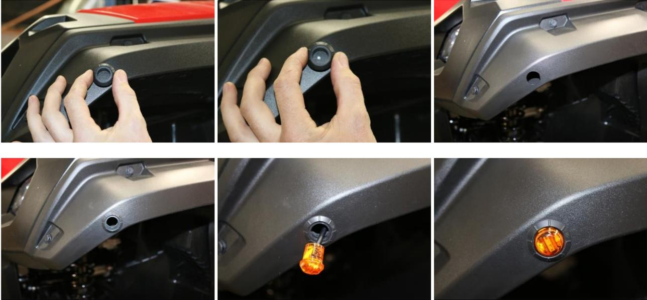
Insert the grommet into the hole, take the wires from the LED and insert into grommet, the LED has a TOP mark on it, insert it into the grommet with the TOP up.
