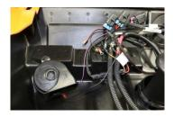
Connect the violet wire to one of the horn terminals and the black wire provided to the other terminal, run the black wire over to Buss Bar and attach to ground. If the car has not been upgraded with the Buss Bar Power Up Kit or Winch Kit, then the black wire will need to be grounded to the buss bar mounting screws
