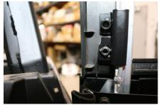
3. Using it as a template, drill the two 5/16" mounting holes, and mount the DRT mirror bracket on the outside.
