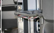
8. Reinstall the door panel and the bottom mirror screw as shown, the bottom screw secures part of the inside door panel
