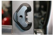
4. Using a marker, mark the indent as shown to drill a 5/16" hole for the wire, remove the mount and drill the hole.
