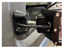
7. Run the mirror wire through the extra hole. Attach 3 wires to the mirror, Red for white light, White for backlight and black for ground. Run the wire down the door to the factory wire harness. Zip Tie the Harness to the factory wires and run to power.
