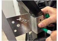
3. Drill the two 5/16" mounting holes and mount the mirror bracket using the supplied bolts and washers.
