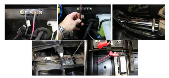
Attach the red cable that was run to the terminal that is marked battery
