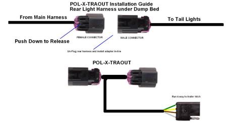
WARNING! Keep the wire Harness away from any hot or moving parts.
