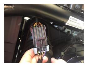
Plug the adapter into both OEM connectors.
