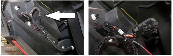
WARNING! Keep the power wire away from any hot or moving parts.
