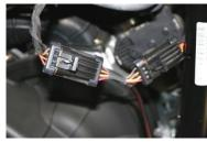
2. Plug the adapter into both OEM connectors as shown above.
