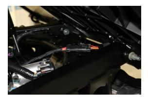
Unplug OEM light connector located under rear dump bed. Plug the adapter in.
