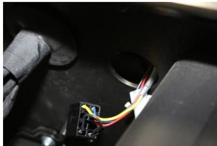
5. Cut out a switch opening in the dash using the supplied template or use a factory switch cut out. Make sure there is room behind the dash for the Switch and Harness
