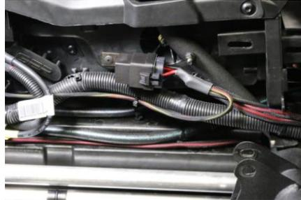
3. The Switch may be mounted in the center dash or between the seats. If up in the dash, remove the plastic panel cover in the center under the dash and run Switch Harness up to one of the factory switch spots and insert switch.
