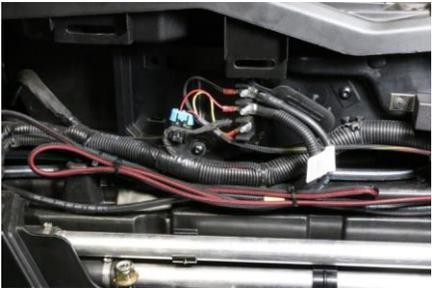
11. Using the supplied cable ties, secure the harness to the vehicle and verify operation.
