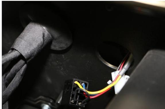
4. Using the provided switch template, mark and cut the dash for the switch, do not over cut. Make sure there is room behind the dash for the switch and connectors.
