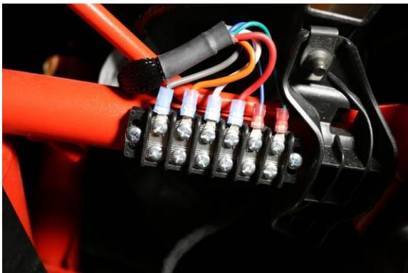
6. Connect the power wire from the devices to be controlled to the appropriate terminal on the barrier strip. Switch 1 and 2 should be used for your larger accessories and are on power relays, switch 3 is for the Strobe circuit and switches 4, 5 and 6 the power goes through the switch and are used for smaller items like whip light, interior lighting, stereo on, Rock Lights, Dune lights, A-Pillar Lights and so on. The following are the switch designations with capacity.
