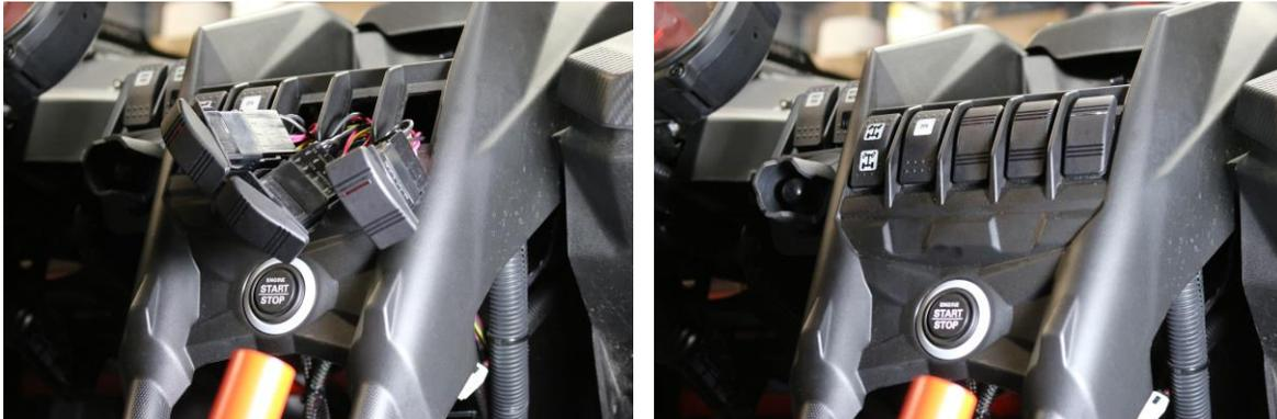
8. Run the other three switches down to the passenger side center console by the cup holders. Attach the yellow wire to the switched bottom stud and the black wire to the top ground stud on the factory busbar
