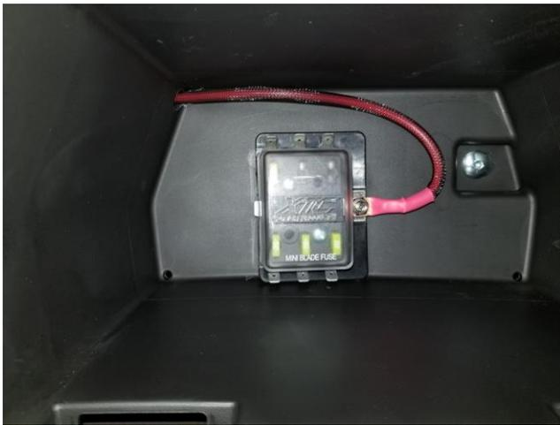
Inside Glove Box - Remove the wires from the fuse block if attached. Mount the Fuse Block inside the rear of the glove box using the #10 self-tapping screws. Drill  $\frac{3}{4}$ " hole in the upper left-hand corner of the box, this can be accessed from the front outside under dash cover. Install the provided  $\frac{3}{4}$ " grommet, insert fuse block wires into glove box and attach to terminals in the following order. Grey to fuse 1, Orange fuse 2, White Fuse 3, Red fuse 4 and Pink fuse 5.
