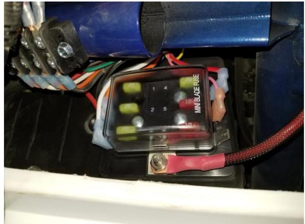
Outside Glove Box - Using the fuse block as a template mark the side of the glove box and drill with  $\frac{1}{4}$ " bit.
