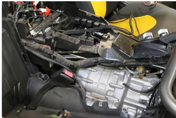
2. Mount the control box on top of the center storage box with the 10-24 x 1/2" machine screws provided.
