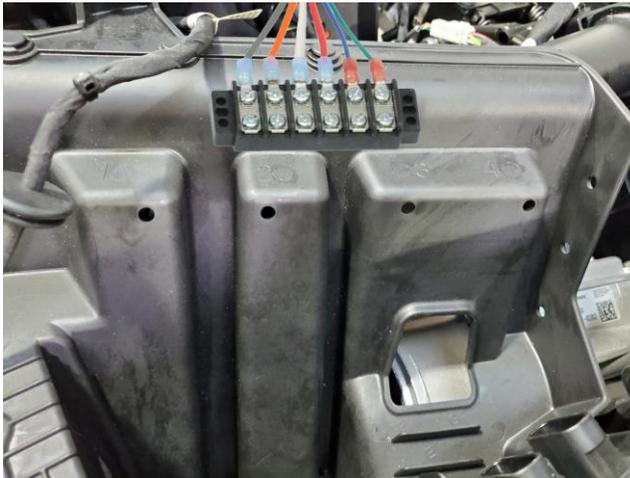
7. Mount the 5/16" Ground Stud – next to the Terminal Block. Run the 8GA Black cable from the 5/16" stud to the center Negative stud on the Factory Busbar. Use the provided 5/16" Ring terminals to attach grounds to each device.
