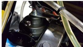
3. From underneath the dash run violet wire through the fire wall to the horn.
