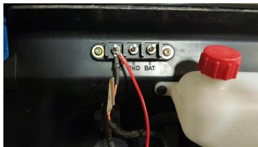
Newer RZR Busbar's have Battery and Ground attached.
