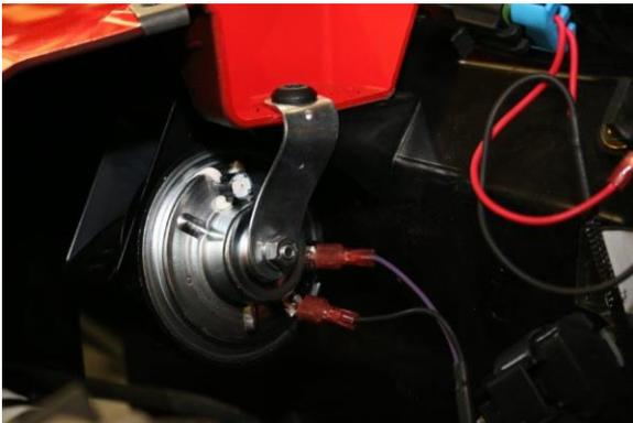
3. Connect the Black wire to the other horn terminal and ground. Remove one of the bolts attached to the frame and install the ground wire under it. It can also be hooked to the ground on the factory Busbar if the Busbar has a Battery Ground Cable.
