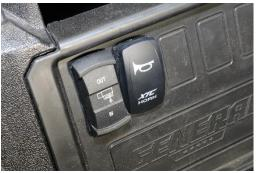
7. Remove one of the blank plugs from the factory Busbar and plug our horn connector in.
