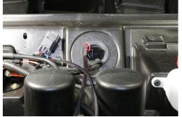
5. Cut out one of the switch mounts and run the 8-pin connector through the cutout
