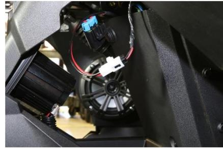
5. Verify operation of Horn. Turn Key on and the Bottom Switch LED should illuminate, Push the top of the Horn Rocker and the Horn should sound.
