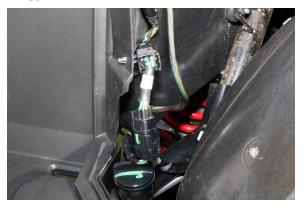
WARNING! Keep power wire away from any hot or moving parts.
