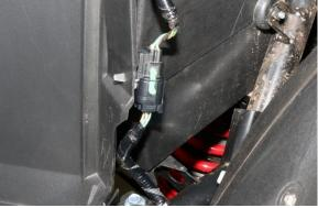
3. Unplug that connector and plug this adapter inline. If you have our Turn Signal System installed, plugging this adapter inline after will include the signals, before will only give brake out on the Green and Yellow wires.
