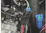
2. Next to the Power Steering unit is a blue connector, un-plug the blue connector from the holder by lifting on the small center tab. Plug in the adapter, attach the device to be powered, all devices installed should have there own in-line fuse
