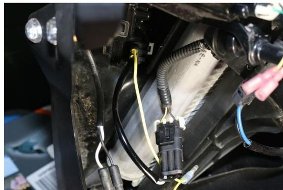
5. **Plug the Turn Signal** – wire into the yellow plug on the adapter. The adapter provides a secondary female bullet connector output for the original signal.
