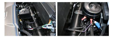
6. Mount Billet Turn Lever – Run the Billet Lever wire from inside the dash to the steering wheel, remove the screw that holds the steering wheel tilt lever, discard the hardware removed, install the lever bolt through the removed bolt hole, make sure to put the new bushing in the center and secure with the included nut. Line Lever housing up and tighten mounting nut. Secure wire harness with included cable ties.
