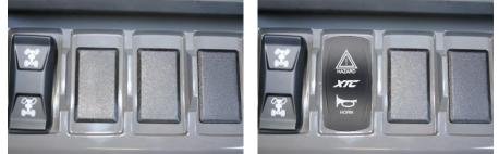
Run Switch Harness–Plug the Switch Harness into the Control Module, run Horn/Hazard connector through the rectangle switch cutout and use included grease on switch terminals then connect Switch and slide into dash.
