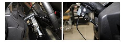
7. Install the Horn/Hazard Switch. Remove 1 of the switch plugs.
