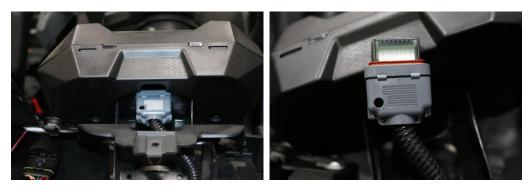
9. Remove Connector Lock – Using a small screwdriver push in on both sides at the white connector shown below and slide lock off.
