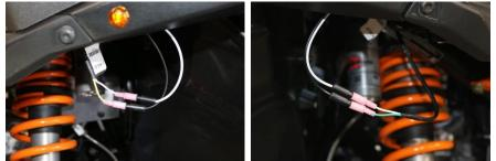
5. Install the Horn. On the front frame under the hood, there are two Torx screws, remove one and mount the horn. Connect the Violet and Black wire to horn terminals, position does not matter.
