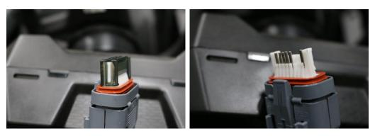
10. Remove Plugs – Using a pair of needle nose pliers remove the plugs from wire port 6 and 7, insert green wire terminal into 6 and yellow wire terminal into port 7.
