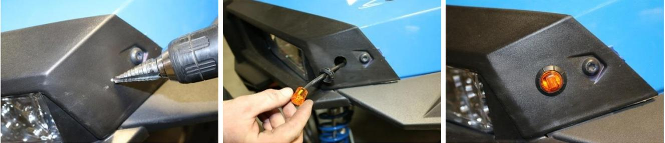
3. **Run the short front harness** from the front LED lights to the control module and plug into mating connector. The Green wire harness go to the right/passenger side and the yellow wire harness go to the left/driver's side. Both green and yellow wires are positive and go to the black wire on each side, the white wire goes to white. Secure the harness with the provided cable ties. **NOTE: Black wire is positive, and the White is ground, they will not work if reversed.**
