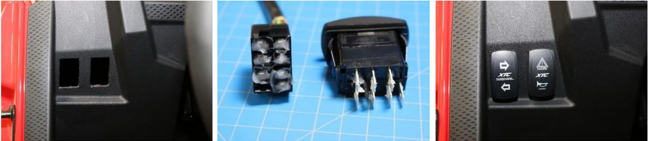
**Dielectric Grease** - Just like the OEM uses on their switches, we recommend using Dielectric Grease on all switch terminals, this keeps the water out, thereby reducing corrosion and helps increase reliability! Open the grease and put on the switch terminals and the connector terminals on both the Turn and Horn/Hazard switches, the more the better.
