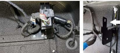
8. Remove the fuse cover and find the 10-amp fuse # F28 as shown and remove.
