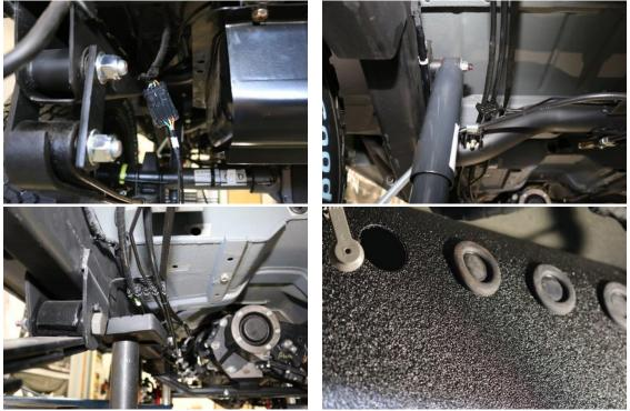
Mount the Control Module as shown below under the grommets using self-tapping screw provided and Plug the Rear Harness in.
