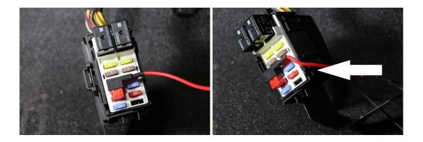
10. Run the power wire down the slot on the right side and reinstall the fuse cover. Remount the fuse box and using the Fuse Mounting screw attach the black ground wire as shown.
