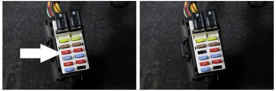
9. Plug the fuse adapter into F28 as shown below.
