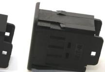
7. Plug the 2-Way power Connector into the Control Module. Run the other end with the fuse over to the fuse block on the passenger side under the dash. To make it easy to work and see the fuses there is a tab on the right side that can be pushed in to release the fuse box, more information can be found in your Instruction Book. Also, it can be removed by removing the 2 screws at the bottom of the bracket, one screw must be removed later to attach the ground wire.
