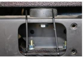
3. Unroll the long rear cable, plug it into the rear harness just installed. Run the cable under the chassis. Remove two Rubber Grommets and using a razor blade cut an x in the center of each one and run the Rear Harness connector through one of the grommets and reinstall in one of the holes. Secure the harness using the supplied Cable Ties.
