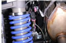
2. Remove the Hood and mount the control unit under the hood as shown using the included screw.
