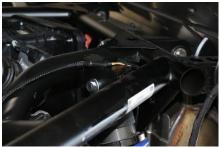
Secure the harness using the provided cable ties.
