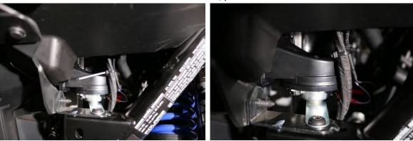
7. Install the Turn and Horn/Hazard Switches. Remove 2 of the switch plugs in the positions you would like to use.
