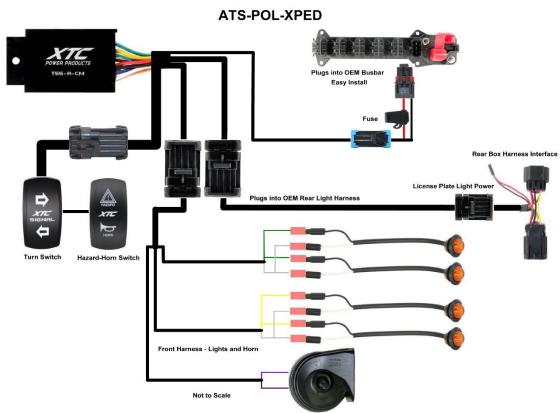
1. Install Rear Light Harness – Lift up the dump bed. In the middle rear over the motor is a 8-way connector, un-plug that connector and install the PPA TS-POL-GTX-REAR harness in line. The 4-way connector should be pointed up.
