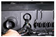
3. Install the extension harness PPA TS-REAR-15EXT. It is run from the rear harness up to under the hood. Remove the drivers' side front fender and side plastics. Plug the extension into the main control unit to verify which direction the harness should go. Push the other end with the female connector (shown above right) into the grommet and feed through the dash over to the driver's side kick panel/fender well as shown below.
