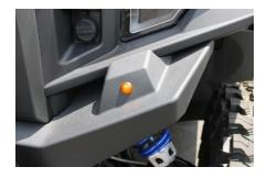
5. Install front wire harness – Plug the harness into the control unit. Run the yellow wires to the driver's side LED's and the green wires go to the passenger side LED's. The wires go under the fender, there is a hole down alongside the headlight that the wires can be run through. We drilled extra holes on each side to help run the wires.
