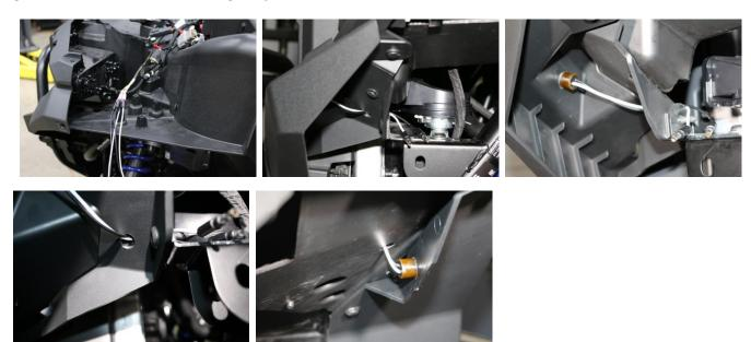
6. Install the Horn. Remove the Torx screw that hold the plastic to the frame in the wheel well. Install the horn as shown Connect the Violet and Black wire to horn terminals, position does not matter.
