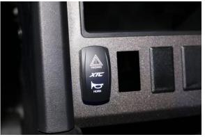
Run Switch Harness—Run the large switch connector from inside the dash, through the rubber grommet and Plug into the Control Module, run the two connectors through the rectangle switch cutouts and use included grease on the terminals then connect to turn switch and Hazard/Horn, slide switches into dash.
