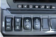
Run Switch Harness–Plug the Switch Harness into the Control Module, run the two connectors through the rectangle switch cutouts and use included grease on the terminals then connect to turn switch and Hazard/Horn, slide switches into dash.
