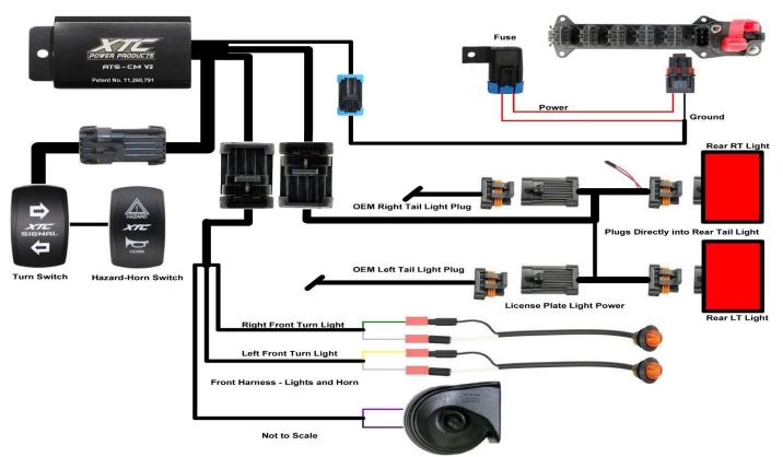
1. Install Rear Light Harness - Take the long rear harness with five connectors and unroll. Remove the 4 Torx T-40 screws holding the bed box. Also remove and the front Hood and Dash Cover, two Torx screws each.
