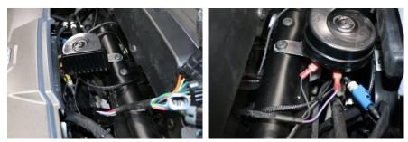
6. Install the Turn and Horn/Hazard Switches. Remove 2 of the switch plugs.
