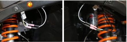
5. Install the Horn. On the front frame under the hood, there is two Torx screws, remove one and mount the horn. Connect the Violet and Black wire to horn terminals, position does not matter.
