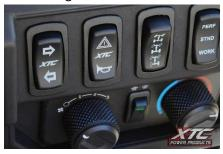
Connect to OEM Dash Indicators - Note: The connector has power in it, disconnect the battery during installation.
