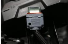
8. Remove Connector Lock – Using a small screwdriver push in on both sides at the white connector shown below and slide lock off
