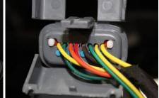
10. Close Cover – Run ATS wires alongside the OEM harness and snap shut, re-install plastic locking cover and plug back in.
