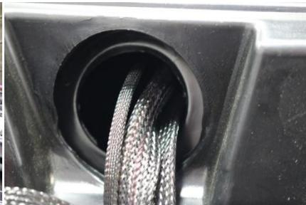
7. Secure rear wire harness making sure to keep it away from any hot or moving parts using the supplied cable ties.
