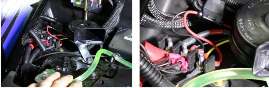
**(Note: The car does not have ground hooked on any of the studs under the hood unless the Bus Bar Power Up kit or Winch kit are installed, the first stud is keyed 12vdc, second stud is ground if wired and the third stud in battery direct if installed, but no fuse or circuit breaker. You must run a ground wire from the chassis to the ground stud or run our black ground wire directly to the chassis for a ground if upgrade is not installed)**
