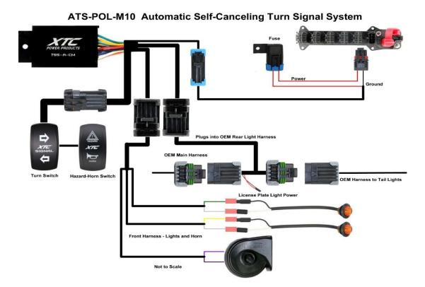
1. Install the Rear Harness - On the rear driver's side above the engine is the OEM rear taillight harness, unplug the 10-Pin
