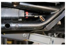
Run along the left side frame from the rear to the front left fender where there is an opening into the dash.
