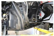
Run the rear harness from the 10-pin connector down along the frame to the fire wall where there is a large wire harness and two small hoses going into the Rocker panel, push the connector through the opening behind these into the side panel.
