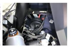
5. Install the Turn and Horn/Hazard Switches. Remove 2 of the switch plugs.
