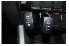
Run Switch Harness–Plug the Switch Harness into the Control Module, run the two connectors through the rectangle switch cutouts and use included grease on the terminals then connect to turn switch and slide switch into dash.
