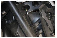
Open the Dash storage and remove the tray, run the harness up into the compartment from the fender.
