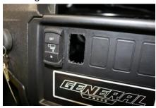
7. Run Switch Harness – Plug the Switch Harness into the Control Module, run the two connectors through the rectangle switch cutouts and use included grease (see step 9) then connect to turn switch and slide switch into dash.
