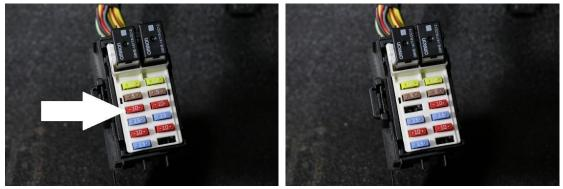
12. Plug the fuse adapter into F28 as shown below.
