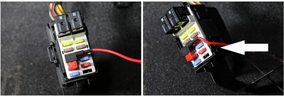
13. Run the power wire down the slot on the right side and reinstall the fuse cover. Remount the fuse box and using the Fuse Mounting screw attach the black ground wire as shown.
