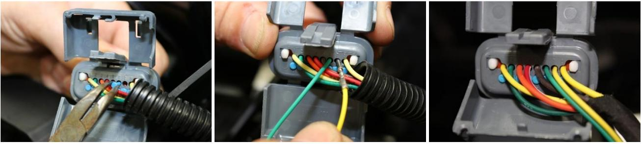
10. Close Cover – Run ATS wires alongside the OEM harness and snap shut, re-install plastic locking cover and plug back in.
