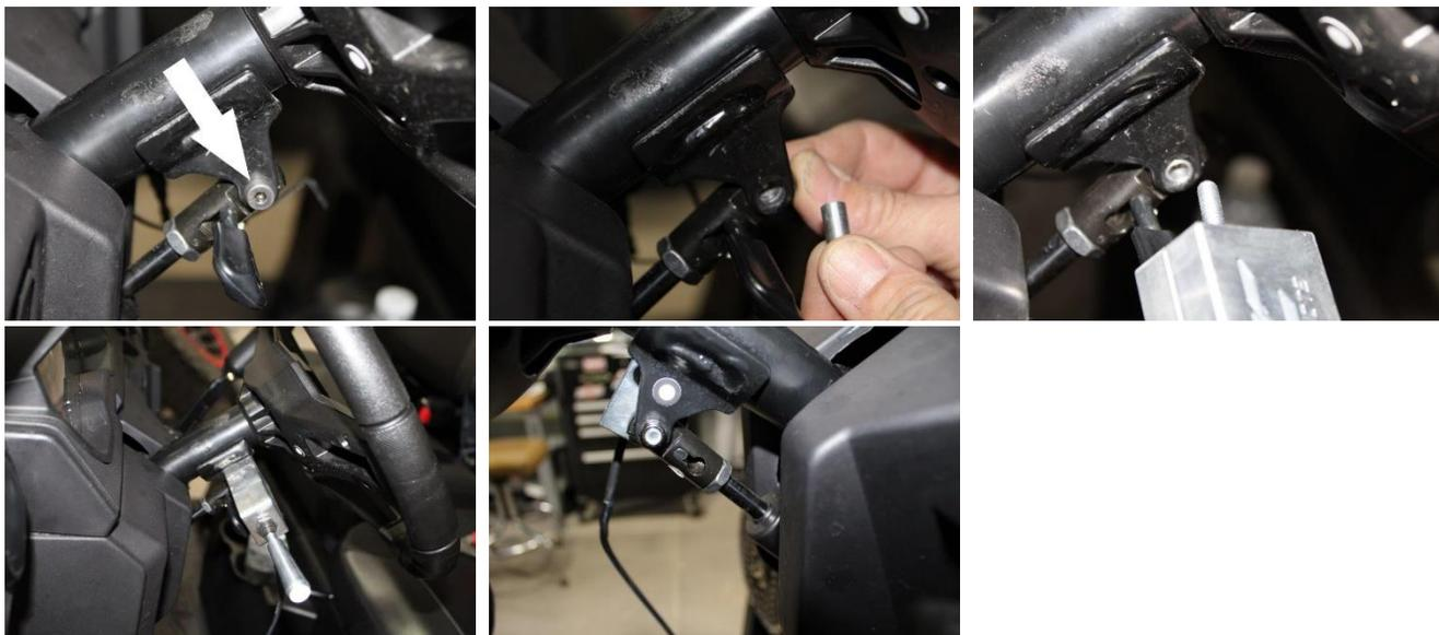
7. Install the Horn/Hazard Switch. On Pre 2021 models, use a new sharp razor, cut switch rectangles out. Do not over cut, try inserting switch and trim as necessary. It helps to rock the razor to cut. On newer models, remove one switch plug. Run the Horn wire connector through the rectangle switch cutout and use included grease on terminals, connect to switch and slide switch into dash.
