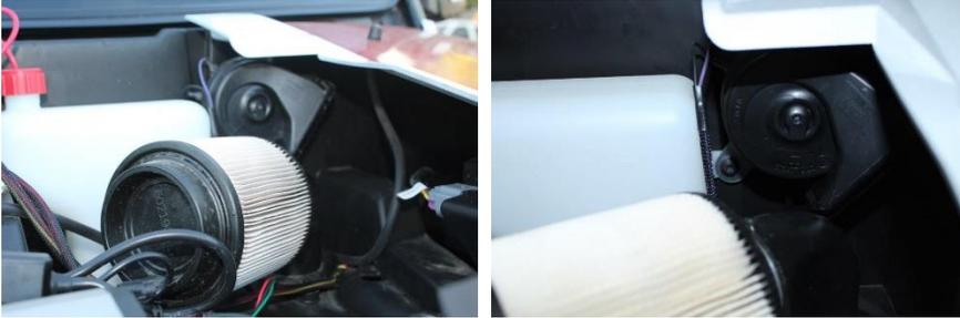
12. Plug the Power Harness into the Control Module. Run the power wire to the Busbar, remove one of the blanks and plug into the Busbar.
