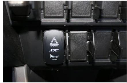
Run Switch Harness—Plug the Switch Harness into the Control Module, run Horn/Hazard connector through the rectangle switch cutout and use included grease on switch terminals then connect Switch and slide into dash. **NOTE:** The switch cut outs are counter sunk, we have supplied 2 switch seals to be used as spacers to keep it raised out of the indent to keep it from getting stuck.
