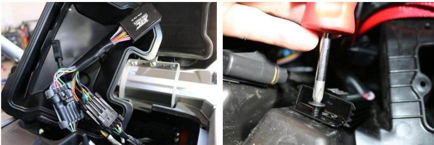
14. Using the provided Cable Tie's secure the harness completely. Reinstall any removed parts.
