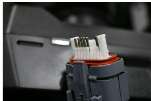
8. Remove Plugs – Using a pair of needle nose pliers remove the plugs from wire port 6 and 7, insert green wire terminal into 6 and yellow wire terminal into port 7.
