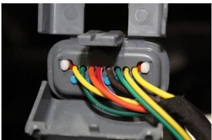
9. Close Cover – Run ATS wires alongside the OEM harness and snap shut, re-install plastic locking cover and plug back in.
