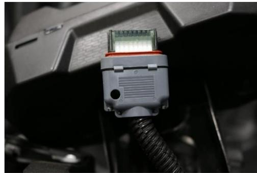
7. Remove Connector Lock – Using a small screwdriver push in on both sides at the white connector shown below and slide lock off
