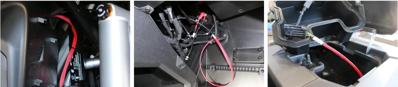
Open the Dash storage and remove the tray, run the harness up into the compartment. Plug into the Control Module.
