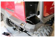
3. Unroll the long extension cable and plug it into the rear harness, run the cable along the frame to the battery compartment, remove the rocker panel and run the cable through the frame up to the control module. Lift up on the floor and feed the cable through the floor at the arrows.
