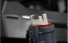
10. Remove Plugs – Using a pair of needle nose pliers remove the plugs from wire port 6 and 7, insert green wire terminal into 6 and yellow wire terminal into port 7.
