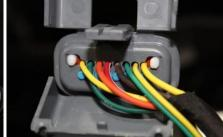
11. Close Cover – Run ATS wires alongside the OEM harness and snap shut, re-install plastic locking cover and plug back in.
