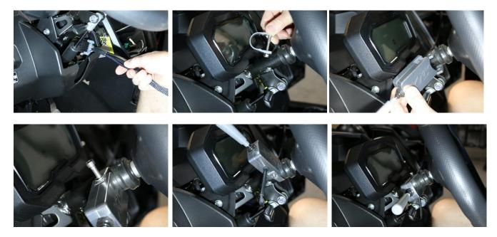
9. Install Hazard/Horn Switch - Install Hazard Horn Switch, using a sharp box knife cut out the rectangle. Push the switch Connector and wires through and apply grease and attach to switch and install in dash.
