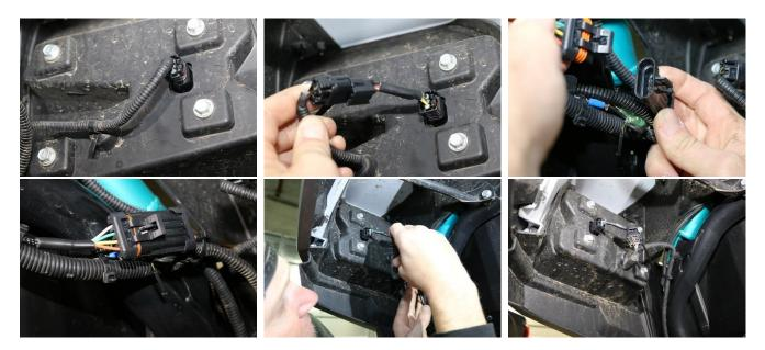
4. Unroll the long extension cable and plug it into the 4-way connector that was just installed from the 4-pin connector down to the rear fire wall through the rubber grommet with the other cables behind the driver's seat, go across to the center console and run alongside the shifter up to the control module that was installed in step 2 and plug in. Keep it away from any HOT or MOVING parts. Using the provided Cable Ties secure it to the main OEM wire harness
