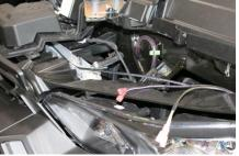
Run the other end with the 4-pin connector to the center cubby where the rear harness was run.
