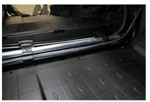
3. Run the Rear Extension Harness –Unroll the Long Extension Harness and plug into the new rear harness. Make sure to keep the harness away from any HOT or moving parts, run the other side with the 4-pin connector down through the opening that leads into the center tunnel, unlatch the cars cable harness's and insert our harness up to the center dash opening. Secure using the supplied cable ties.
