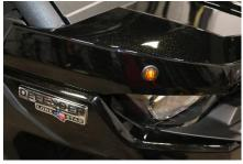
7. Attach Front Harness to lights - The Green and white wire go to the right/passenger side LED, attach the Green to the Black and the White to the White, the Yellow and white wire go to the Left/Driver side LED, attach the yellow to the Black and the white to the White. NOTE: Black wire is positive and goes to the Green and Yellow wire, they will not work if reversed. White is ground. Pull any excess wire back under the dash and secure the Harness using the provided cable ties.
