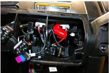
13. Verify operation of all lights. Cable ties any extra harness under dash. Reinstall center tunnel.
