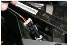
Remove both rear taillights by removing two bolts from the side of each one using a #10 Socket. Run the rear harness along the OEM harness, slide the heat tubing to the same spots as the factory reflective heat shield and cable tie in place. Continue attaching to the OEM cable, the green wire goes to the right-side light and the yellow wire goes to the left-side, cable tie at the same points as the OEM harness, plug each light in and reinstall taillights.
