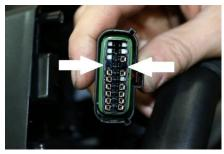
Insert the green connector wire into port 7, insert the yellow connector wire into port 17.
