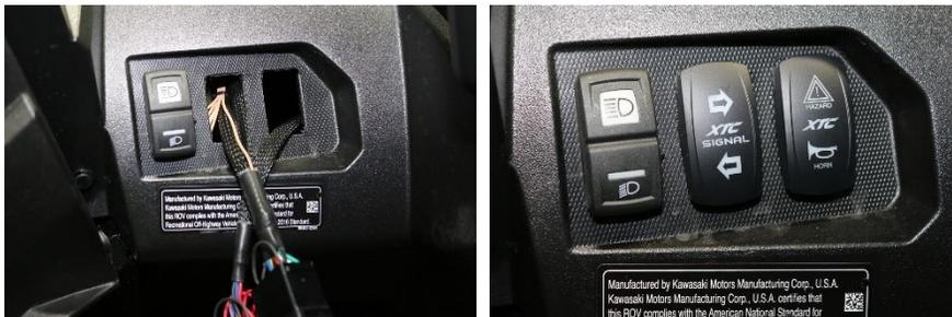
**Dielectric Grease** - Just like the OEM uses on their switches, we recommend using Dielectric Grease on all switch terminals, this keeps the water out, thereby reducing corrosion and helps increase reliability! Open the grease and put on the switch terminals and the connector terminals on both the Turn and Horn switches, the more the better.
