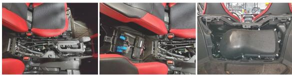
2. Using the provided Self Tapping Screw mount the Control Module under the hood on the bar as shown. Since it is small and light it can also be strapped to the main power harness with the included cable ties.
