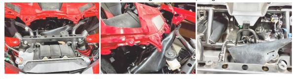
Remove Center Console Plastics and Rear Box Cover to run rear harness.
