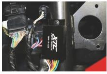
3. Unroll the Rear Harness. Next to the air cleaner, unplug the 6-Way Connector (shown with white arrow) and Plug the rear harness in-line. There is a Black and Red wire provided for power to an optional License Plate Light.
