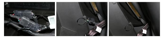
4. **Run the other end** - of the rear harness to the front kick panel. The plastic has a perforated circle behind the driver's seat or rear seat behind the driver on the MAX, at this location you can push the rear harness single connector through the plastic gap to the passenger compartment, follow the frame along the driver's side, the harness can be hidden in the side panels and goes up behind the removed kick panel and plug it into the mating connector on the Control Module.
