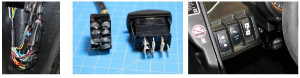
**9.** Install Hazard/Horn Switch - - Remove one of the switch blanks and run our 10-pin switch connector through the opening, grease the terminals with the supplied grease and attach to Hazard/Horn switch and insert the switch into the opening.
